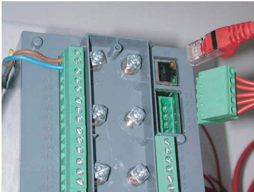
Unplug the RS485 and RJ45 cables
