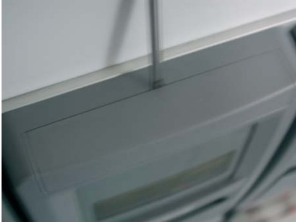
Removing tile to access the fastening screws
